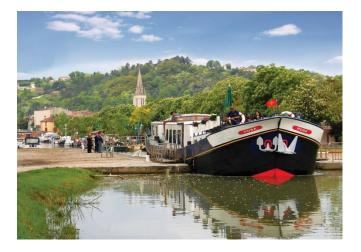
Former purpose:Clipper, built in the Netherlands,<br/>formerly sailed the Dutch SeasYear of construction:1907Dimensions:98ft long x 16ft 4"wide (29.5m x 5m)Generators:2 x 220 volts generators 9 Kw/h and 17 Kw/hMain Engine:Deutz SA6M512 120HPMaximum Speed:4.3 KnotsWater & fuel capacity:5 tons of water and 3 tons of fuel
