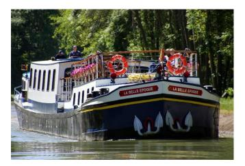
Former purpose: Ex Freight Barge carrying logs from Burgundy to Paris and Amsterdam Year of construction: 1930 **Dimensions:** 126ft (38.4m) x 16ft 6ins (5m) Year converted into a hotel barge: 1995 Generators: 2 x 220 volt generators (silent night) for airconditioning and heating & silent inverter Main Engine: 150 HP M.A.N Maximum Speed: 10 knots Water & fuel capacity: 12 tons of water & 3 tons of fuel
