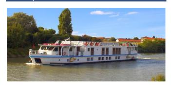
Former purpose: Sand barge on the River Po Year of construction: 1960 21.6ft x 147.6ft (6.6m X 45m) Dimensions: Year converted into a floating hotel: 2010 Generators: AIFO IVECO SRM55M (550 Horse Power x 2) Main engine: Maximum speed: 10 knots Water capacity: 20,000 litres 12,000 litres Fuel capacity: Cruise distance: 174km
